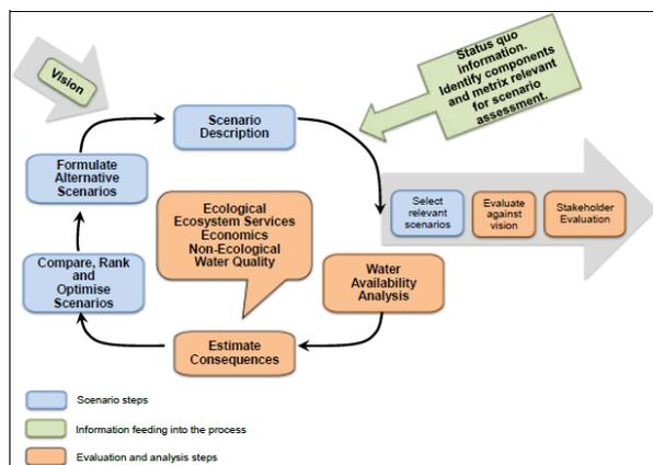
**Figure 1: Schematic representation of scenario analysis process**
